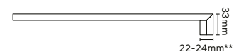
step tread "L" corner . nez de marche "L" angle ecke stufenplatte "L" . degrau "L" canto
